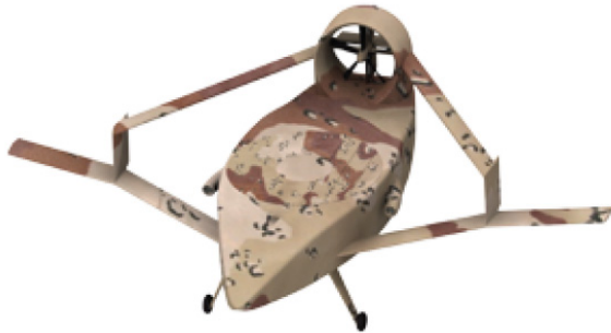
Figure 8 – Wingtip Extensions Attached to V-STAR™
